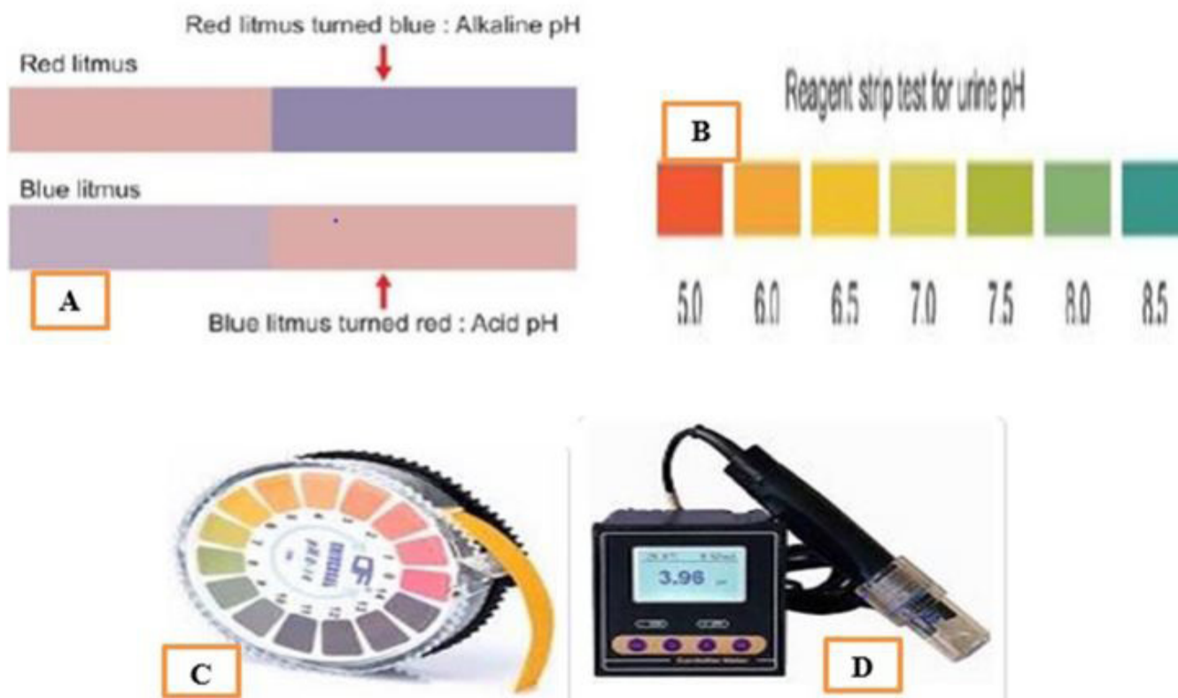
(A) Litmus paper, (B) reagent strip test, (C) pH indicator paper and (D). PH meter
